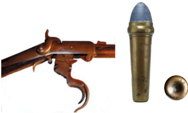
Here is a look at the distinctive breech lock, along with the cone-shaped cartridge that Ambrose Burnside also invented.
